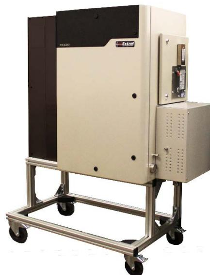
**Figure 5.** The MAX300-RTG, real-time mass spectrometer. For refinery flare compliance, the analyzer is often configured with a Hazardous Area Certification and corrosive-resistant materials that perform well with high-level H<sub>2</sub>S and HF acid, according to site requirements.
